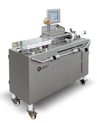
Sausage linker is intended for formation of frankfurters and small sausages of the same length by twisting 16-36 mm artificial polyamide, cellulose, collagen casings followed by transfer to forming table or hanging device for further hanging on smoking stick by the molding operator. The range of products is limited to meat raw materials of industrial animals, poultry, fish with temperatures from -4 °C to +20 °C. Fillers KOMPO, Vemag, Handtmann, Frey, Rex can be used as pressure pump.
